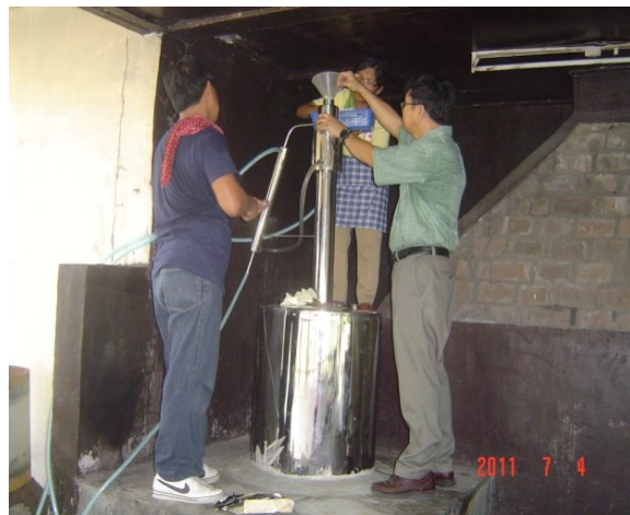
Fig. 2. Design A. 241L capacity equipped with unmodified cooling system from manufacturer’s design.
