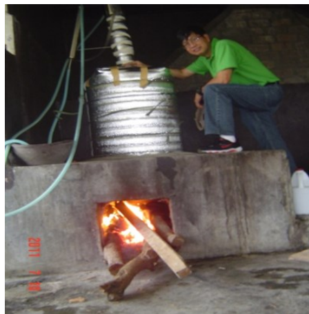
Fig. 3. Design B. 241L Capacity equipped with unmodified cooling system with insulator.
