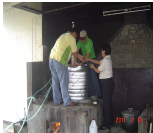
Fig. 3. Design B. 241L Capacity equipped with unmodified cooling system with insulator.
