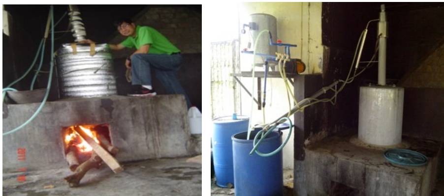
Fig. 5. Design D. 241L Capacity equipped with insulator and modified cooling system ( proposed optimized design ).
