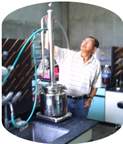
Fig. 2. Design A. 241L capacity equipped with unmodified cooling system from manufacturer’s design.
