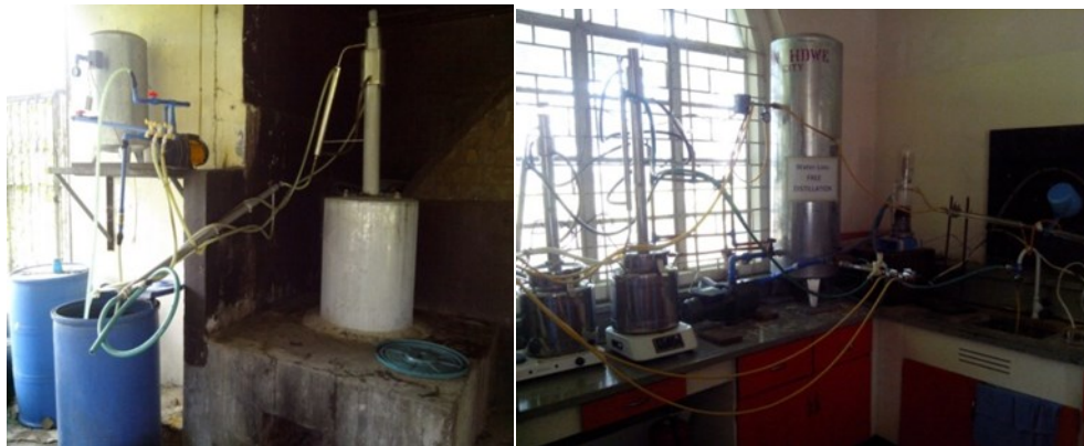
Fig. 4. Design C.1. 241L Capacity equipped with modified cooling system (at CRL). C.2 .3-in-1 distillation system (at CAS).
